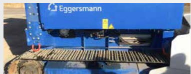
For increased traction on loose ground – the landfill undercarriage
