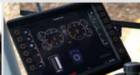
Control via touch panel
