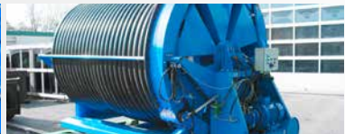
BACKHUS HD S, Radio controlled – hose drum with 3" or 4" connection
