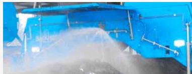
Process optimization – injecting water during turning
