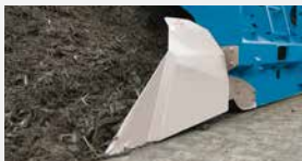
Ground adjusting track clearers
