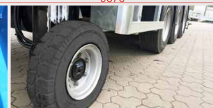
Drive unit – allows to move the machine using the radio remote (Semi-trailer only)
